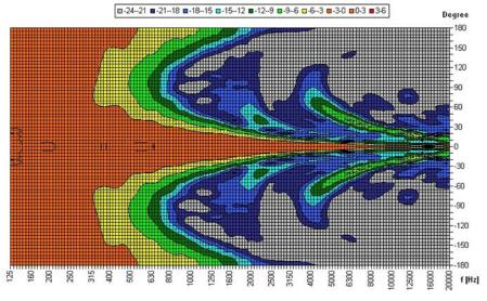
Parameters: Cyclic Move:  $0^\circ$ ; Symmetry: average sym; Freq.Smooth: 1/3 Oct; Ang.Resol.:  $5^\circ$ ; Rel. to:  $0^\circ$ Axis  $0^\circ$
